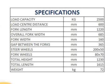
With fork dimensions of 685x1220mm, this wide pallet truck model is aimed at those using UK or the larger Chep pallets (100x120cm or 120x120cm) - but it can also pick up the common Euro pallet (120x80cm) from the long side.
